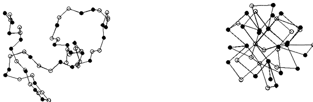
Figure 5. Snapshots of the chain configuration at the temperatures ( N = 60 ). Solid circles correspond to hydrophobic and open circles to hydrophilic residues respectively. T = 3.85 (left) and T = 1.00 (right).
